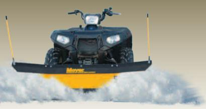
The dual flared wing moldboard design coupled with the 65° attack angle, provides scoop and funnel discharge action.
